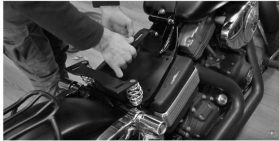
Pin the shorter bolts on the battery side, and the long ones on the other side then tighten them all
