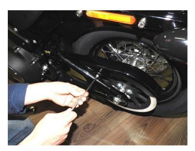
Apply the support on the swing arm tube and secure it with the provided bolt
