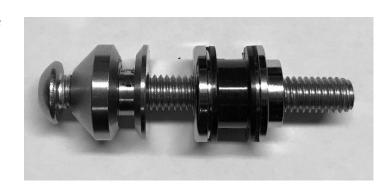
2. **Blinker side:** long bolt + detachable system bushing + sissy bar hardware
