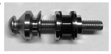
**2.Blinker side:** long bolt + detachable system bushing + spacer + sissy bar hardware
