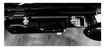
Secure the saddlebag to the motorcycle by sliding its bracket on the bushings, then lock it.
