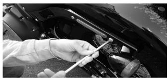
Install the new bolts and bushings provided with the installation kit. (on motorcycles equipped with detachable sissy bar, please use the bolts available in the labeled kit)
