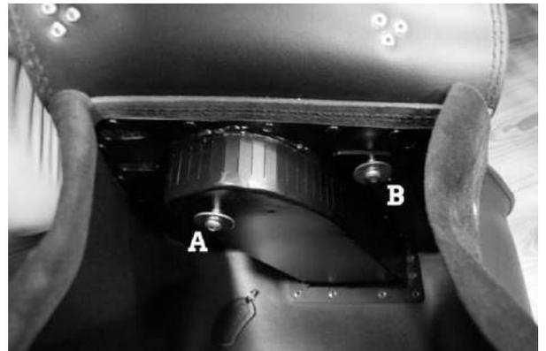
Apply the washer and the spacer on bolt A, then apply the washer, the short spacer and the sissy bar bushing on bolt B
