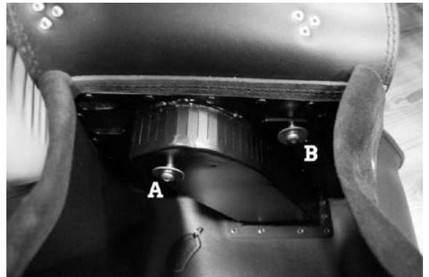
Apply the washers and the spacers on the bolts, and screw the bolt A to the Suspension bolt and the bolt B to the fender
