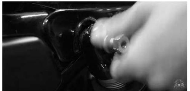
Unscrew the fender bolt
