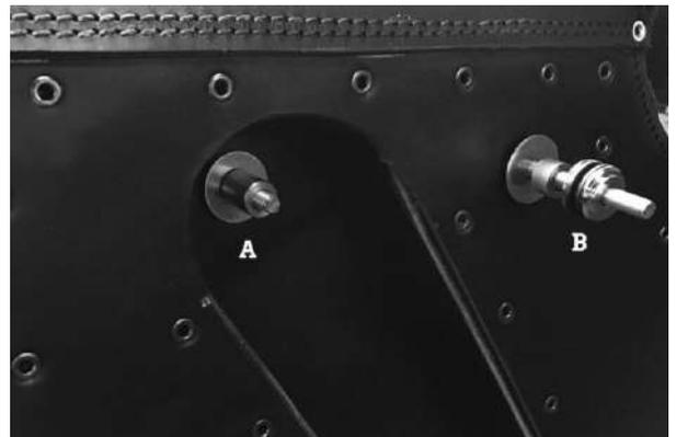
Screw bolt A to the Suspension bolt and bolt B to the fender
