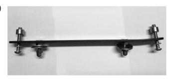
Once installed, place washers on the bracket
