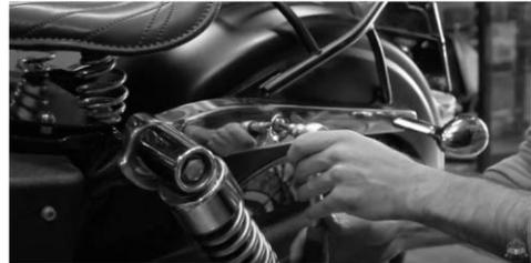
Untighten the turn signal in order to create enough space for the bracket to slip in between the fender and the turn signal itself.
