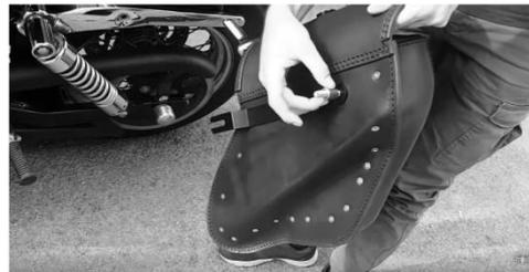
Insert the bracket between the turn signal and the fender
