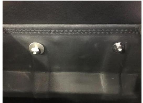
The bolt, included in the installation kit, that has the smaller washer goes outside the bag
