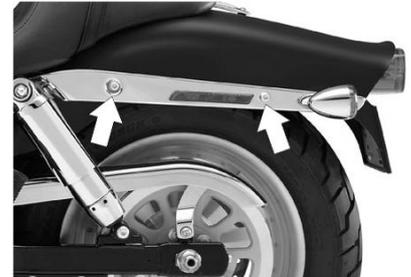
Insert the provided bolts and washers inside the holes in the bag pack panel
